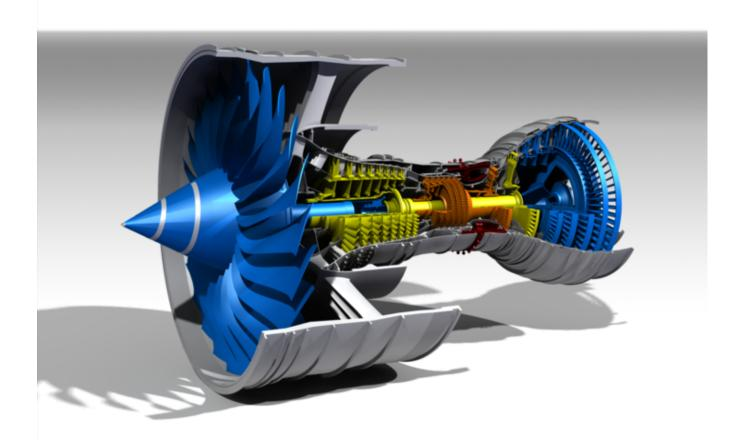
Pratt and Whitney is going with the geared fan approach. Similar to turboprops, there is a gearbox to allow the fan to spin at a lower speed than the engine spool that is driving it.
