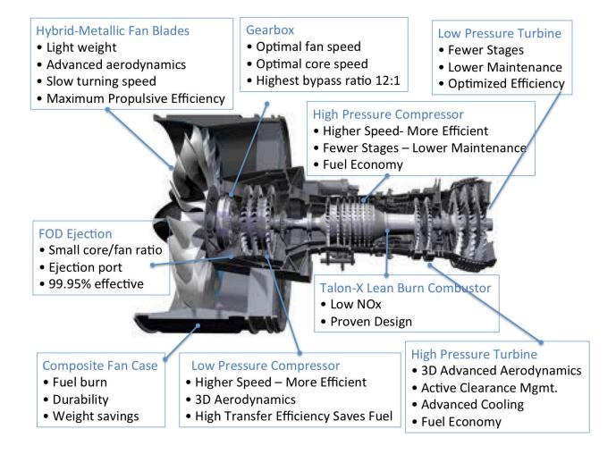
This allows the turbine spool to operate at a more optimal RPM while still allowing the fan to spin more slowly. A slower fan can be larger, allowing for a higher bypass ratio.
